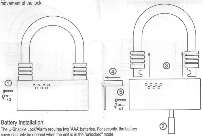
cover can only be opened when the unit is in the "unlocked" mode. (1) Unscrew the external battery cover retaining screws.
